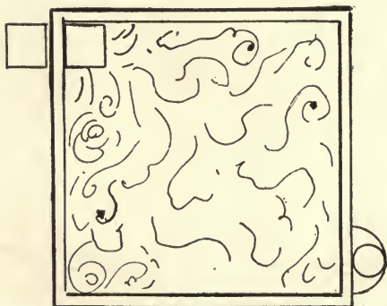
Fig. 192. Movement of water in the same trap under the normal discharge of water. Water from the fixtures it serves.
